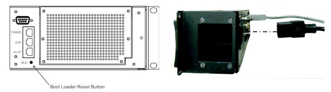
3. While the BLR button is pressed, connect the **power cord** to the keypanel. *KP 32 CLD - Boot Loader Waiting for download... appears in the display window.*
